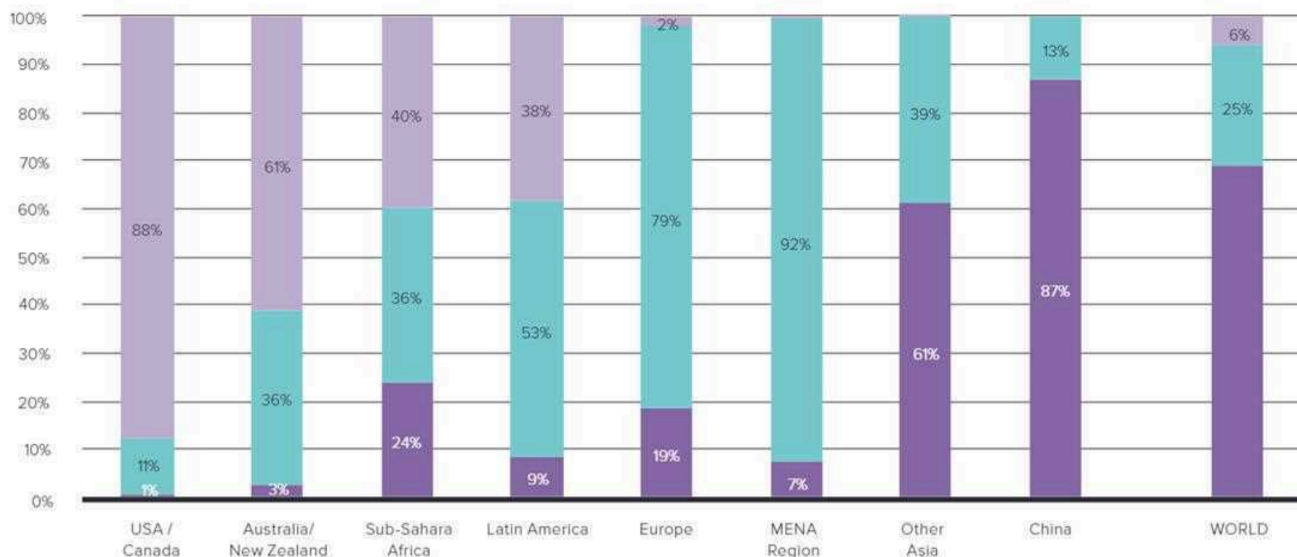
Figure 48: Distribution by type of solar thermal collector for the total installed water collector capacity in operation by the end of 2022
